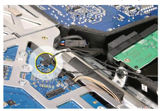
2. Peel back the foam gasket on top of the hard drive. Remove the sensor cable from the sensor clip.
